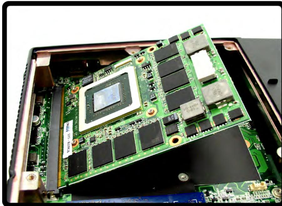
2. The card needs to be fully into the slot, and the video card and socket have a guide-key and pin which align to allow the card to fit securely.
