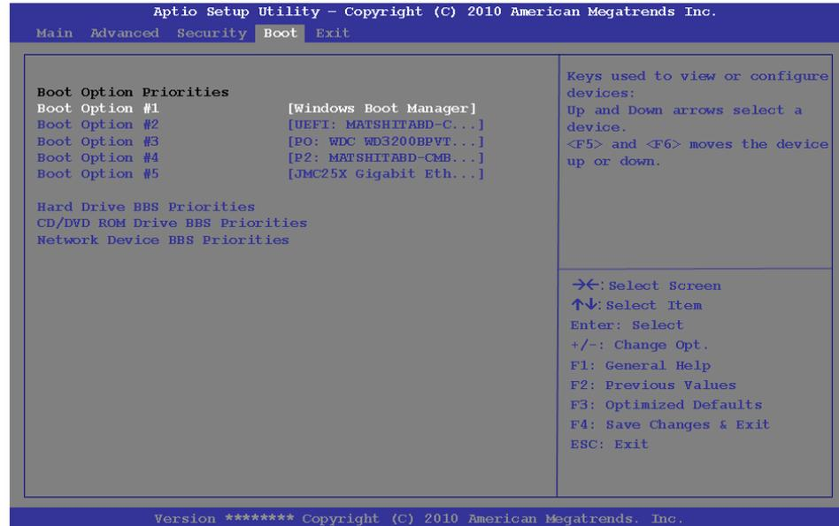
When you turn the computer on it will look for an operating system (e.g. **Windows 7**) from the devices listed in this menu, and **in this priority order**. If it cannot find the operating system on that device, it will try to load it from the next device in the order specified in the **Boot priority order**. Item specific help on the right is available to help you move devices up and down the order.
