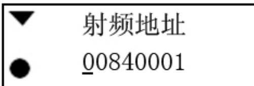
The number underlined is needed to be changed ,pressing 【FEED】 button means to be plus one ,pressing 【MODE】 button means underline moves once on the right;when moving to the last number ,the underline disappeared .press 【MODE】button again means entering the next setting .
