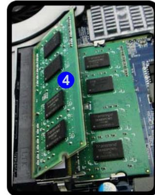
5. Pull the latches to release the second module if necessary.
