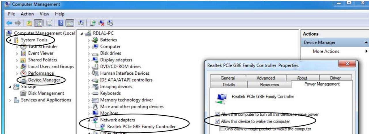
Figure 8 - 6- Network Adapter Wake On LAN (Power Management)
