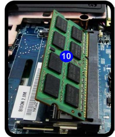
7. Pull the latches to release the second module if necessary.
