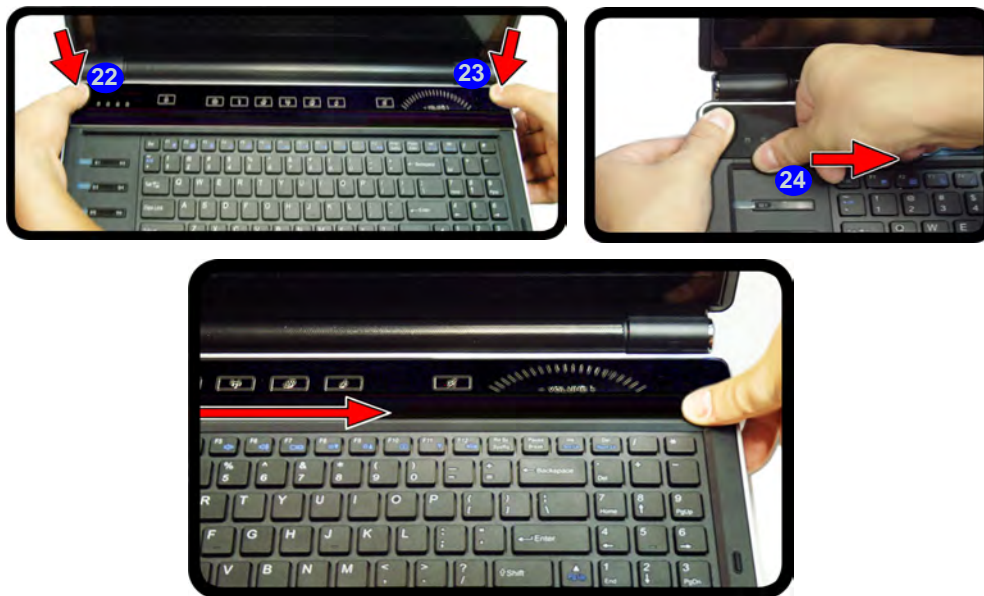
Figure 6 - 20 LED Cover Module Slide to the Right & Snap Down
