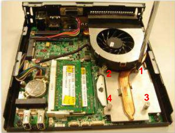
4-1-2. The fan power cord plugged MB, Make sure the direction of fan cable accord the photo
