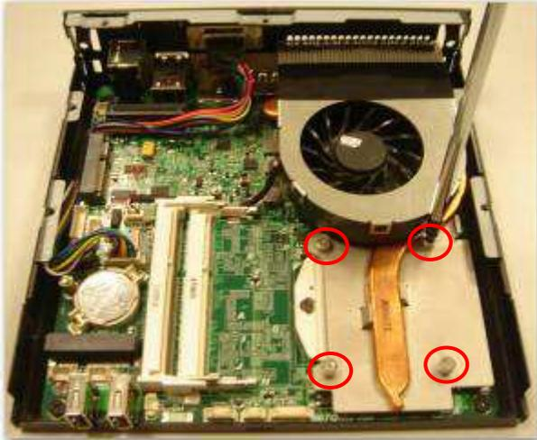
2-1-2. Remove the cooling fan modules and remove the power cord from MB
